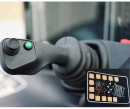
The multi-functional handle provides precise control over key vehicle functions, including forward and backward travel speed, side shifting, and proportional lifting and lowering.
