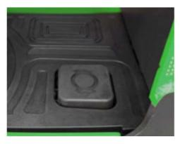
The dual-brake/presence pedal system enhances safety by preventing the forklift from moving unless both pedals are pressed.
