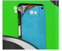
Large capacity battery for multiple shift operation.
