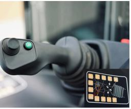
The multi-functional handle provides precise control over key vehicle functions, including forward and backward travel speed, side shifting, and proportional lifting and lowering.
