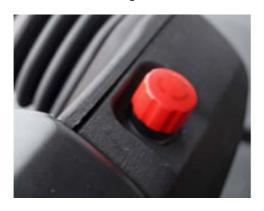
The emergency power button instantly disconnects power in critical situations, ensuring the safety of both the operator and the cargo.
