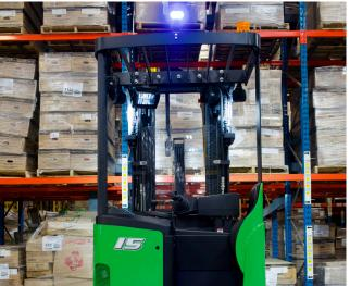
The cab design, open-view mast, and overhead guard provide the operator with a clear line of sight to the load and surroundings, enhancing efficiency and safety.
