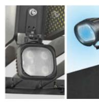
Features LED headlights, a safety blue light, and a buzzer to ensure safe operation while driving.
