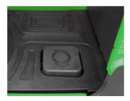
The dual-brake/presence pedal system enhances safety by preventing the forklift from moving unless both pedals are pressed.
