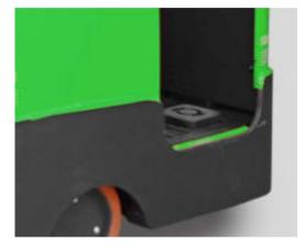
The floor suspension system adjusts to the operator's weight, reducing impact and vibration for a smoother ride.
