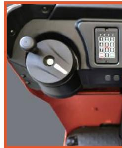
The steering wheel is located under the left hand, giving another solid support position for an operator, which is important for high speed trucks.
