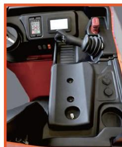
The elbow support has manual adjustment of angle, allowing operators of different height having different length of arms to find comfortable position which would support them during work and keep the solid body position.
