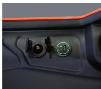
The USB charging socket allows to power and charge mobile devices during the work. Those devices can be placed in the related storage areas with convenient access and securing the devices from falling out during turning, acceleration or braking.
