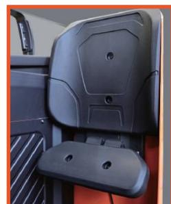
The height of the backrest for operator is electrically adjustable by means of the button located on control panel. The angle of seat support is manually adjustable (default configuration) or electrically adjustable (option) at the same time the seat support is linked with the backrest and can be adjusted for operators of different height too.
