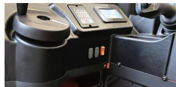
The blue spot light allows to indicate for people around the approaching truck which is increasing the safety.
