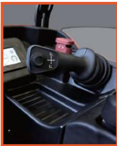
The control joystick with perfect ergonomics is used as operator hold position and located under right hand, the driving, lifting/lowering operations are controlled by thumb, the horn function is controlled by a finger without interruption of driving functions and change of grip position.
