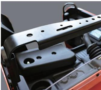
The truck is equipped with mounting bar in front part, allowing to locate various accessories on it (scanners, screens, fleet management and control systems, etc.).
