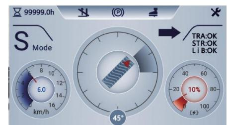
The colored LCD screen, located in front of operator, allows to control major truck parameters, like speed, level of battery charge, position of the steering wheel, currently active speed driving mode, status of electrical systems of the truck (traction, hydraulic and lithium battery) and amount of working hours.
