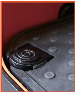
The OPC (operator presence control) switch is made in a form of pedal located on the left side of the operators platform, making sure that feet of the operator are safely located within the footprint of the chassis during driving.
