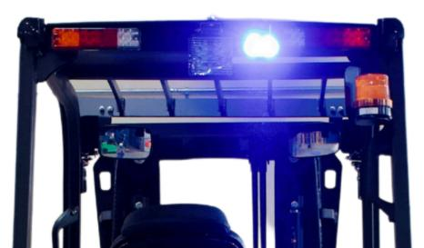
Equipped with LED lamps, rear work lights, headlights, strobe and safety blue light.
