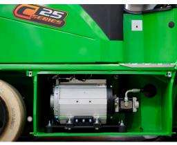
Removable side panels allow for easy service and maintenance, while offering strong protection against water and dust.
