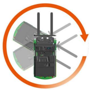
The compact design allows for a 360 degree zero-turning radius, enabling the truck to operate in confined spaces.
