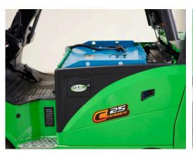
The battery compartment features a side removal assembly for quick and easy battery replacement.
