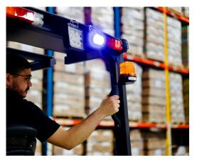
Rear grab bar with integrated horn allows for easy horn access while reversing, while keeping the operator's hand safely inside the truck at all times.
