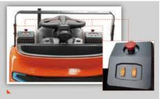
The jog button on both sides of the truck allows the operator to operate truck forward/backward or lift the fork while walking beside. There is no need for the operator to get in and out of the truck frequently to operate it. That greatly improved the picking efficiency and operation safety by reducing the speed controlled by the jog button.
